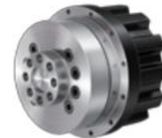
GH 69-980 Nm 10.74-31.43 • Solid shaft • Backlash 6 arc.min. • High speed
